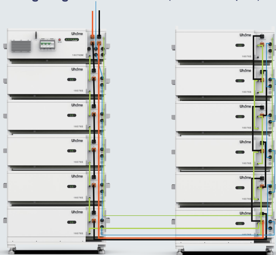
Wiring diagram for 12 units (divided into 2 piles)
